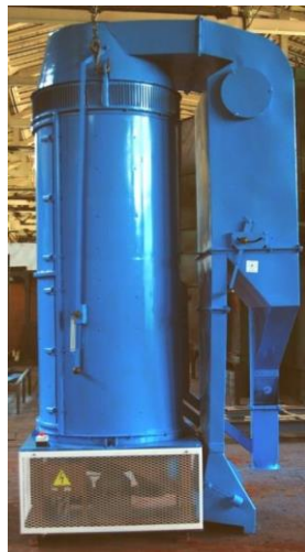
Fig. 1. General view of the combined air separator
